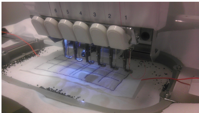
Fig. 1. Encapsulated carbon cathode preparation
